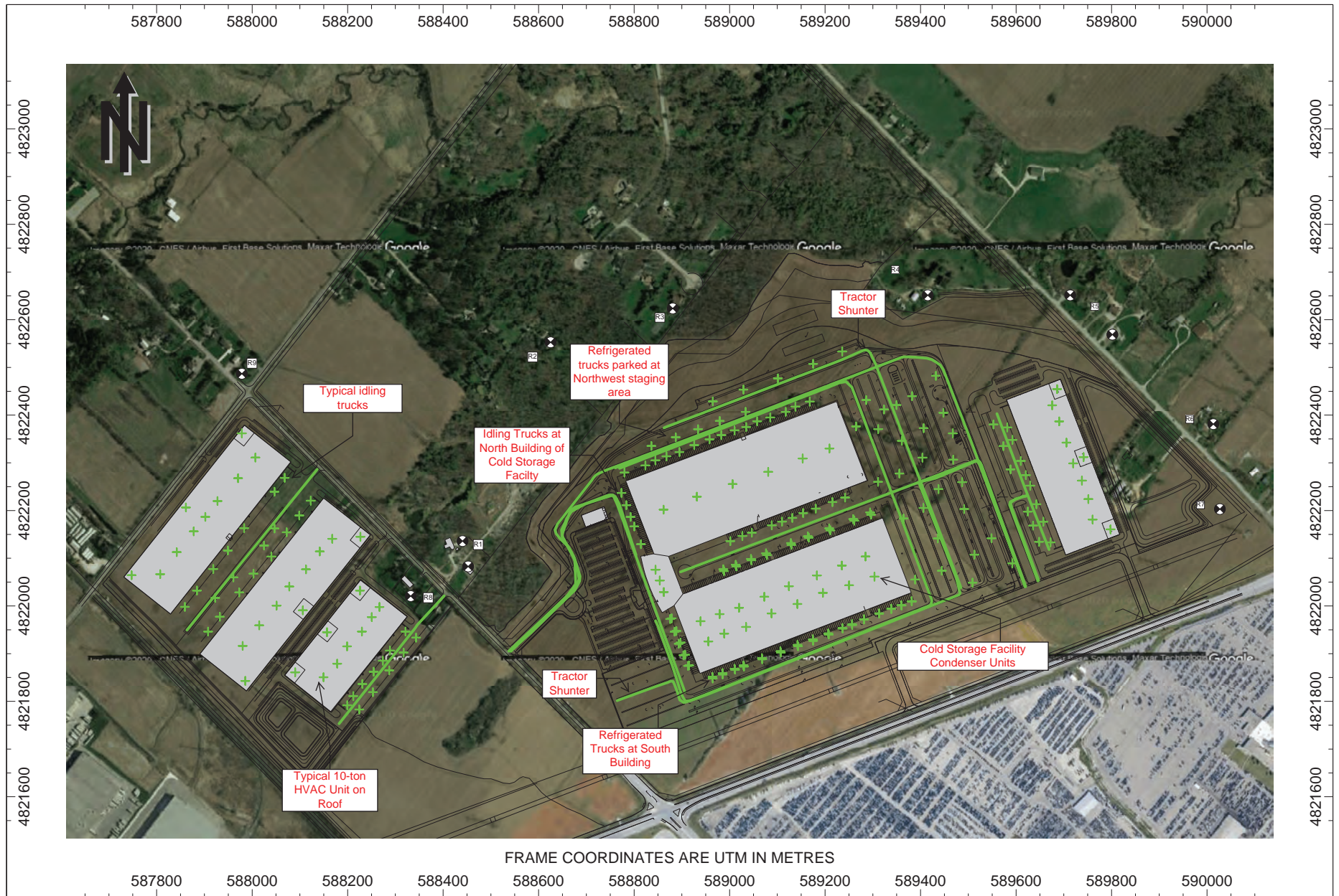
Figure A2: Noise Source Locations
