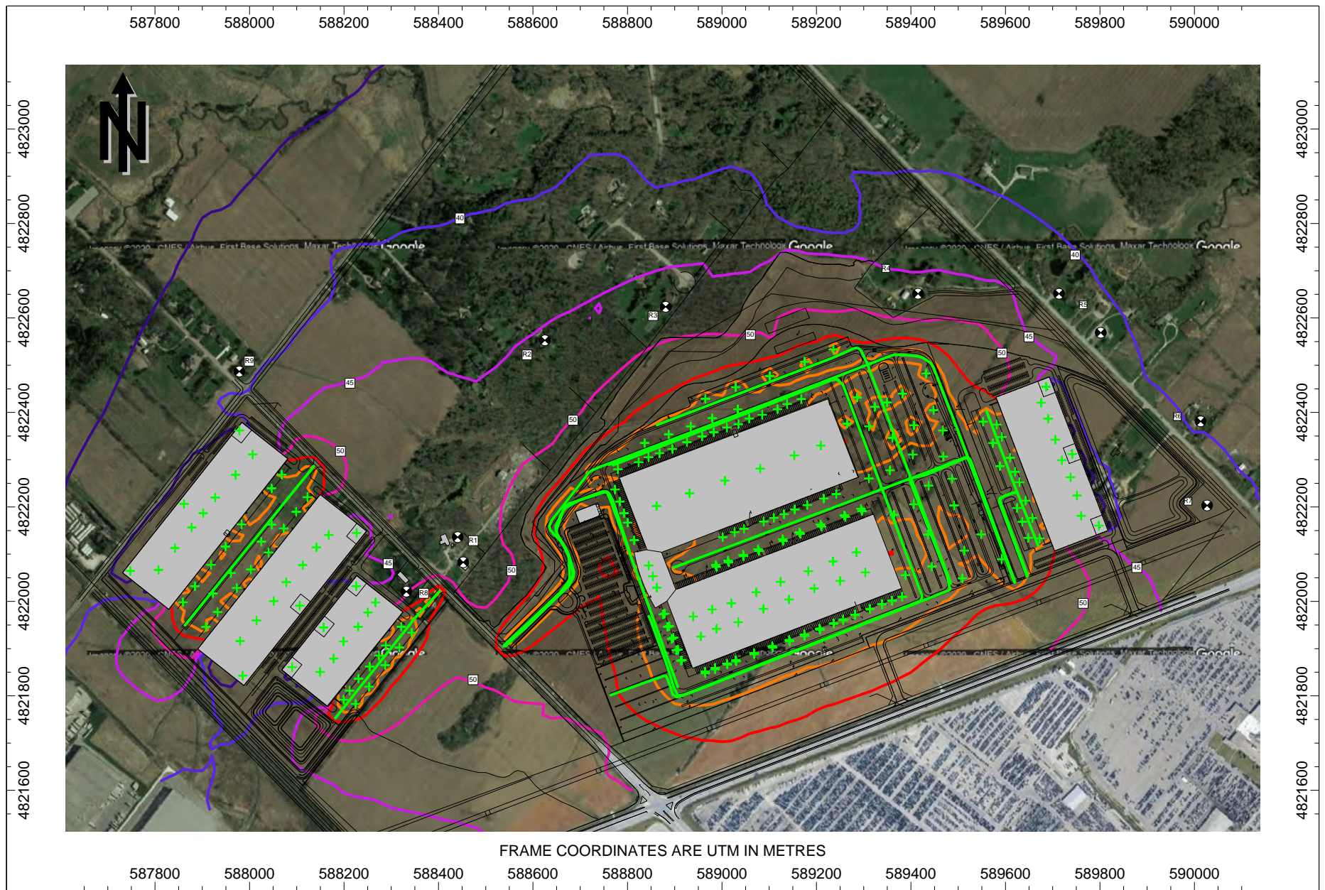
Figure 3: Predicted Daytime Hour Non-Impulsive Sources Sound Level Contours without Mitigation, LEQ1hr [dBA]
