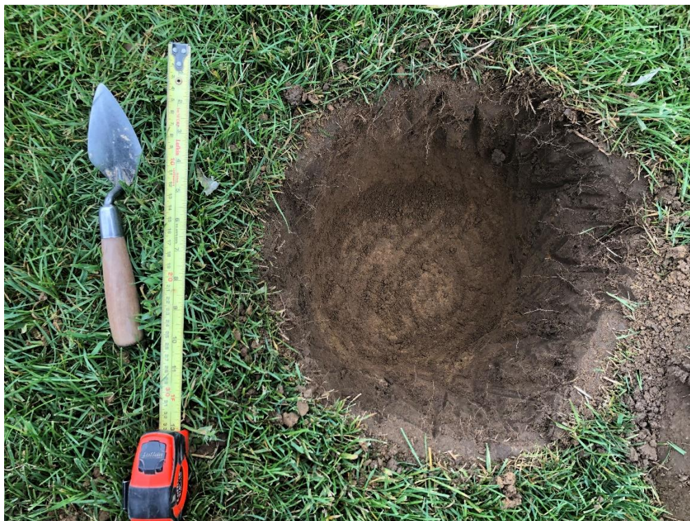
Image 18 Typical test pit stratigraphy for grassed areas tested on a 5 m interval.
