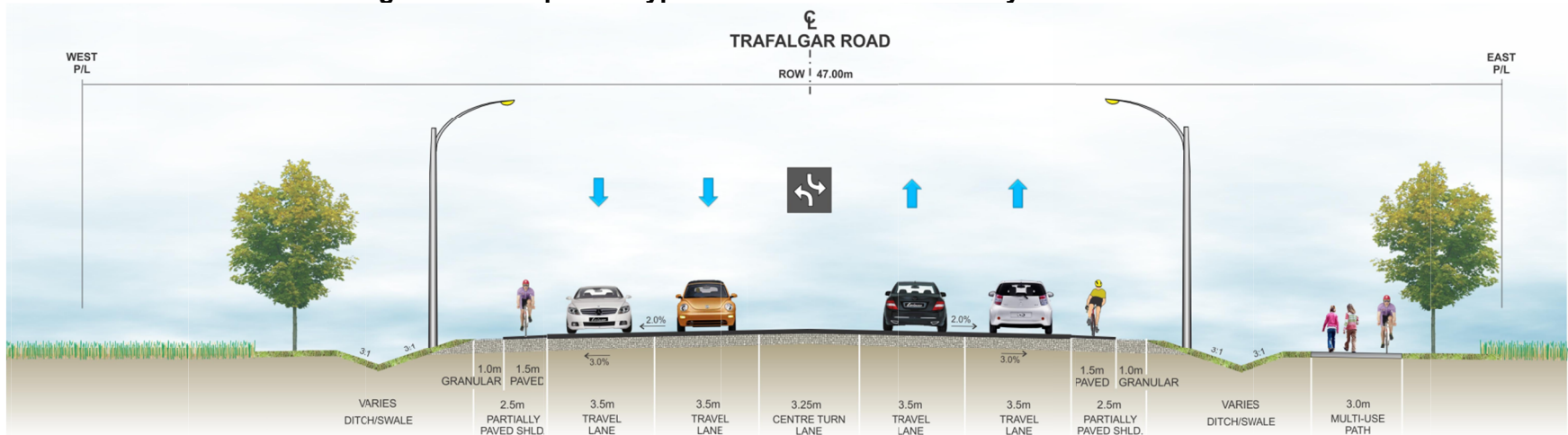
Exhibit 7-2: Trafalgar Road Proposed Typical Cross Section - Hornby Road to North of 10 Side Road
