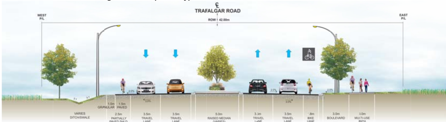
Exhibit 7-1: Trafalgar Road Proposed Typical Cross Section – North of 10 Side Road to 15 Side Road
