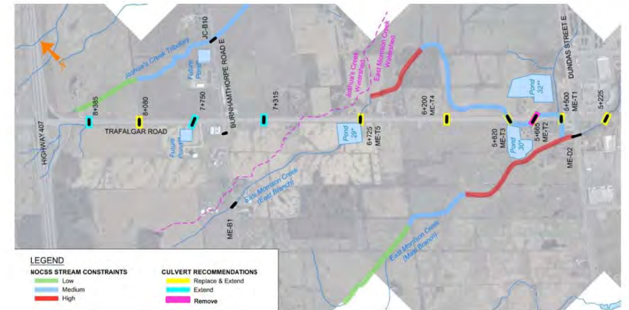
Figure 3.18 Proposed Culvert Replacements, Extensions and Removals
