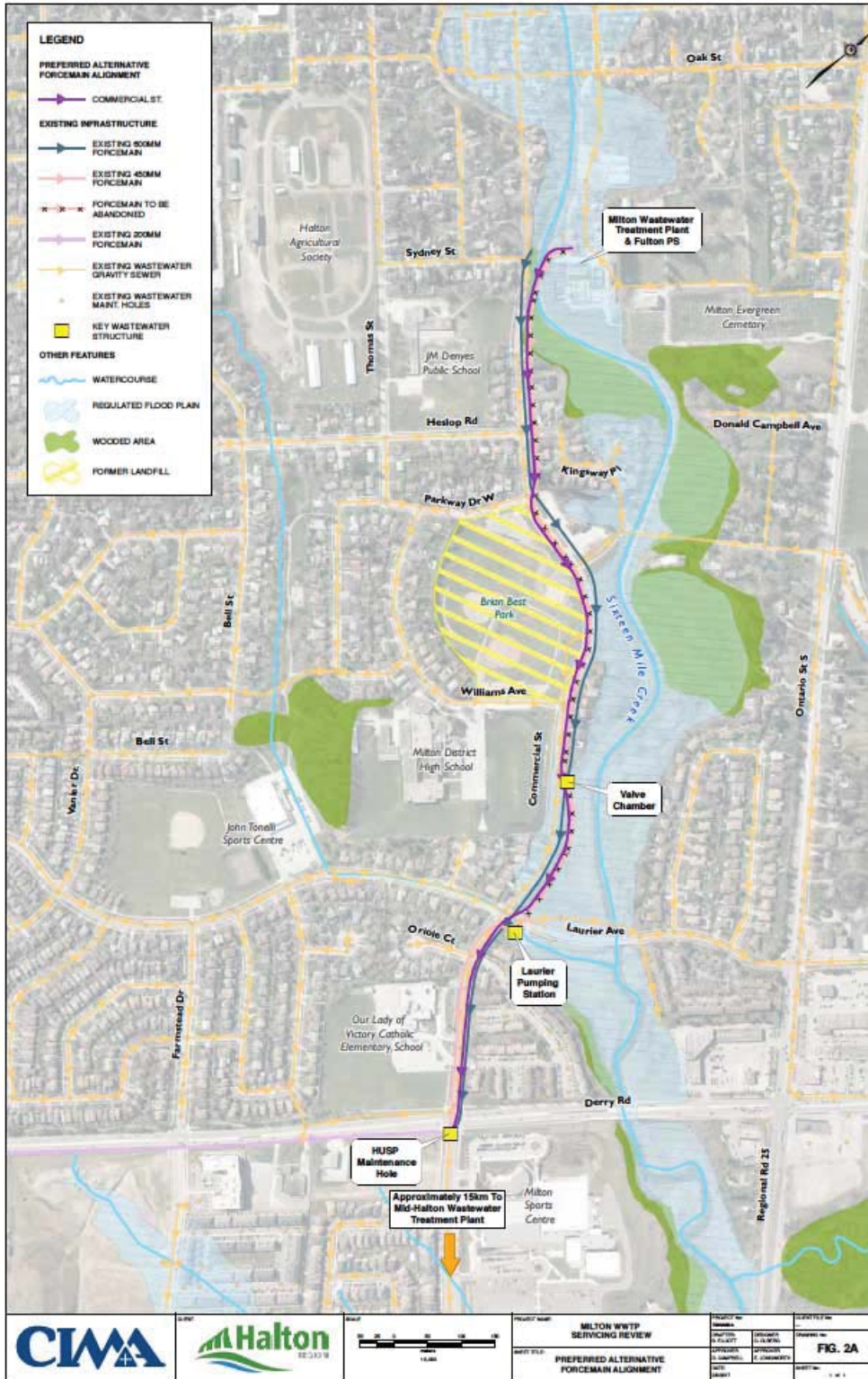
Figure 2. This map shows the Preferred Forcemain Alternative - Commercial Street From Fulton Street Pumping Station to Derry Road and Santa Maria Boulevard, Town of Milton [CIMA+, February 2016].
