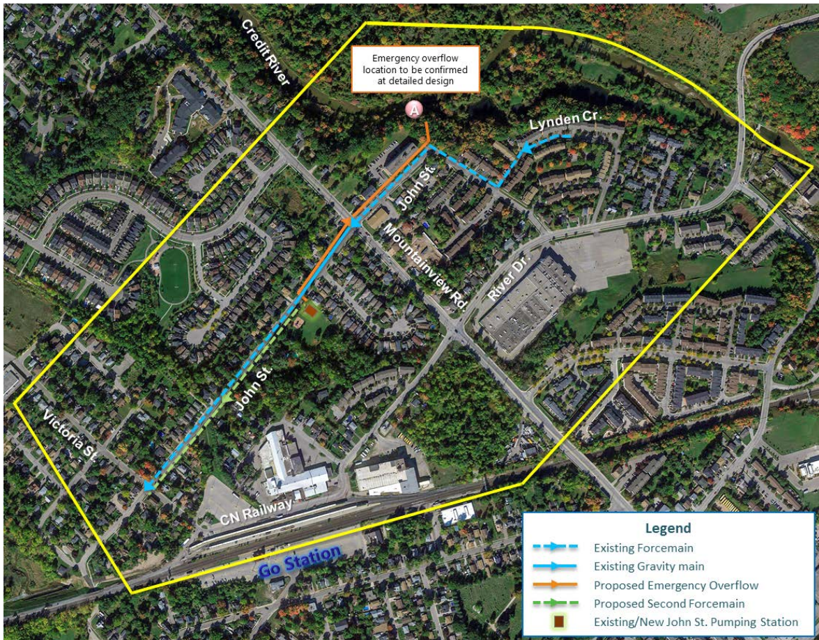
Figure 8: Alternative 2 – Upgrade Wastewater Pumping Station on Existing Site with Emergency Overflow to Location A
