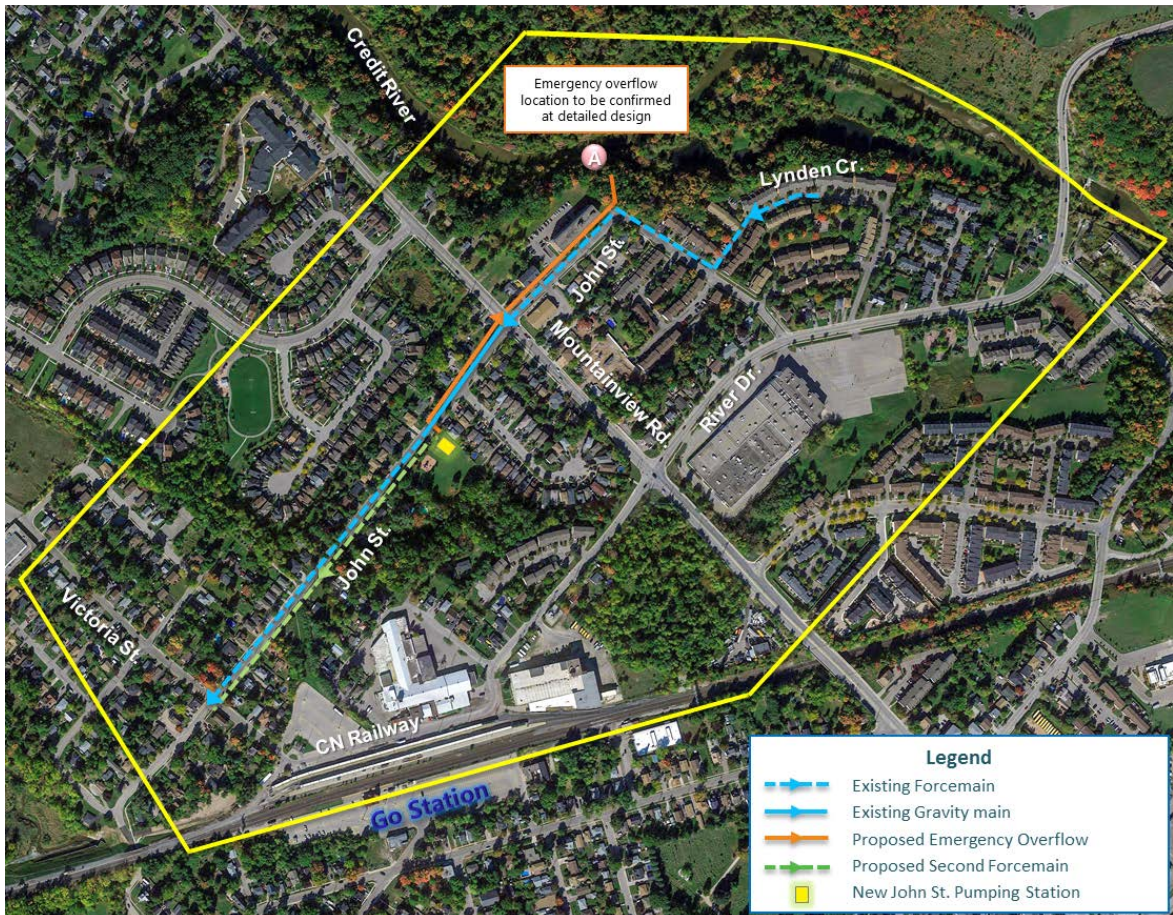
Figure 9: Alternative 3 – New Wastewater Pumping Station on Existing Site with Emergency Overflow to Location A
