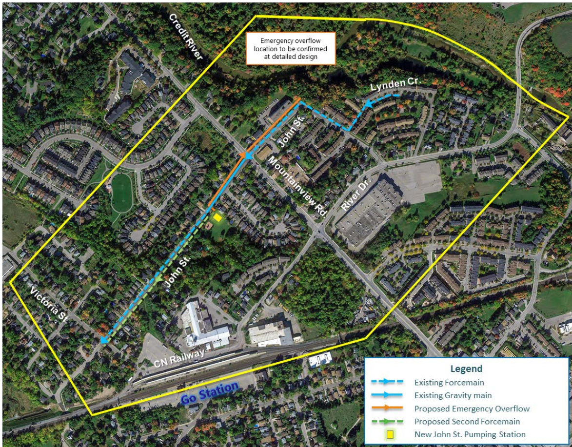
Figure ES-4: Preferred Alternative – New Wastewater Pumping Station on Existing Site with Emergency Overflow
