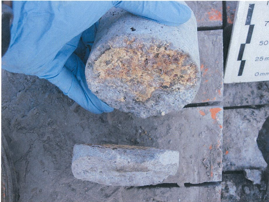
Photograph 13 – Unknown solid substance found in the void of core C24, 70 mm below the concrete surface
