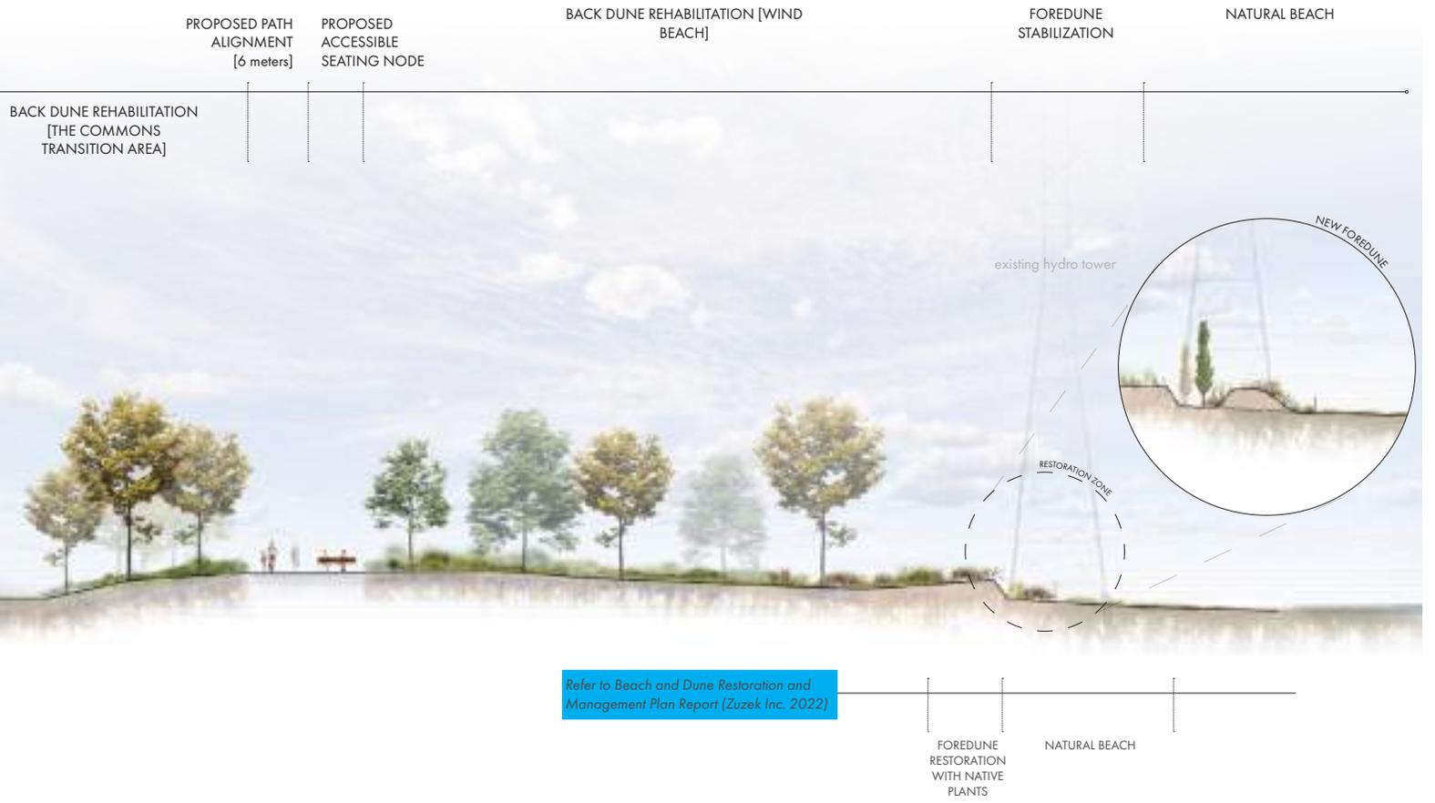
**Figure 3.2.7 - Section of The Commons Transition Area Foredune Restoration and Back Dune Rehabilitation**
