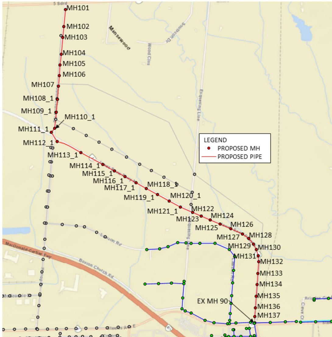
Figure 6-3 New Pipes and Manholes – Option 2
