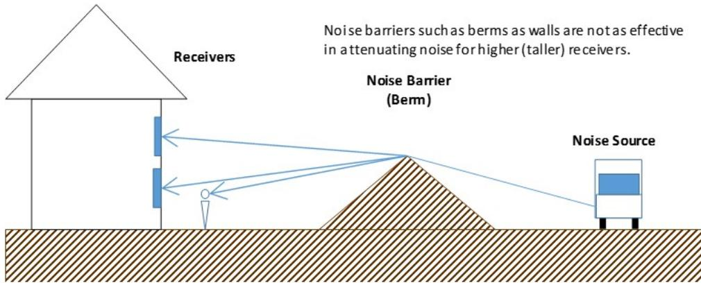
**Figure 9: Effect of Receiver Height on Barrier Attenuation**
