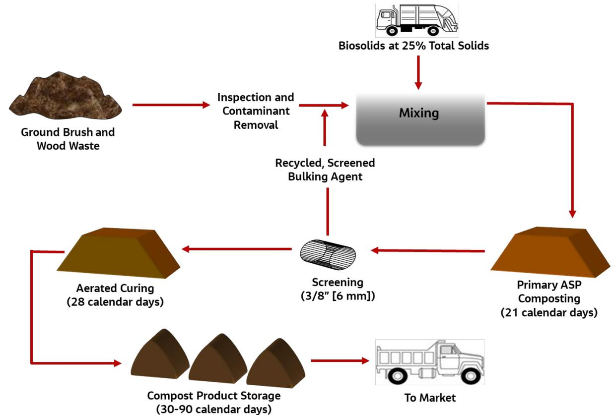
Process flow diagram for a typical ASP biosolids composting facility.
