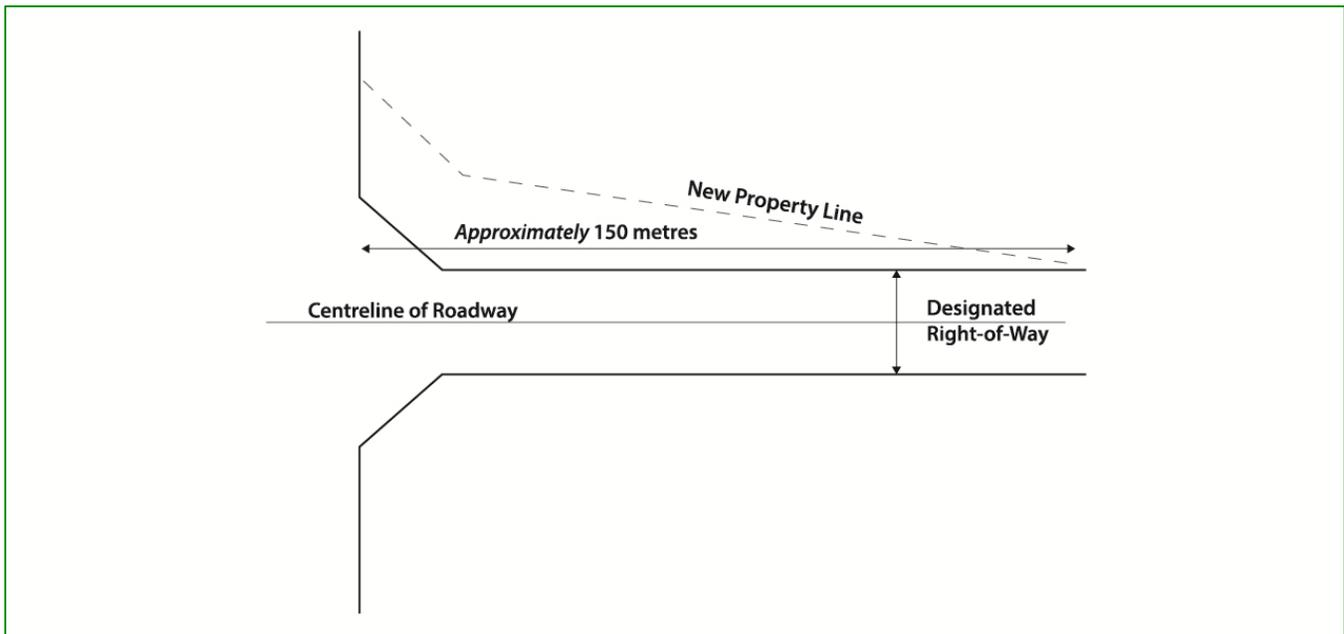
**Figure 1 – Additional Property Required at an Intersection**
