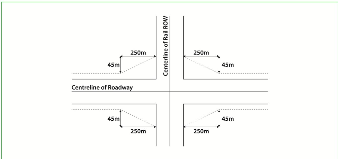
**Figure 2 – Additional Land Required for a Grade Separation**
