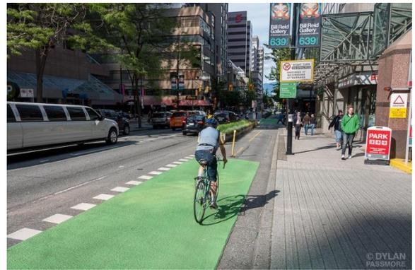
Left-turn queue box: for cyclists making "pedestrian-type" left turn at a traffic signal, and green bike lane through intersection on segregated bike lane, Ottawa ON (photo credit: Citizen Cycle by Ottawa Citizen)
