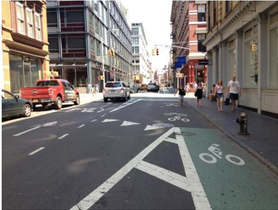
Left-side buffered bike lane approaching a mixing zone for left-turning traffic / cyclists, NYC
