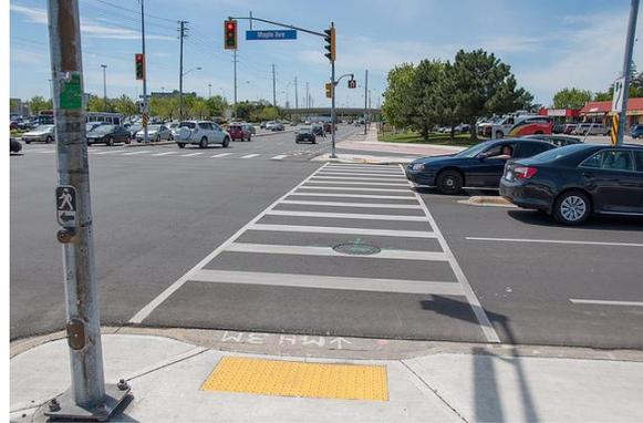
**Pedestrian pushbutton placement:** AODA Regulation 413/2 requires the accessible pedestrian signal push-button to be located within 1.5 m of the curb, a max. of 1.1 m above ground level and 3 m a part if there are two at the same corner). It must be in reach of the accessible sidewalk and near the curb ramp.
