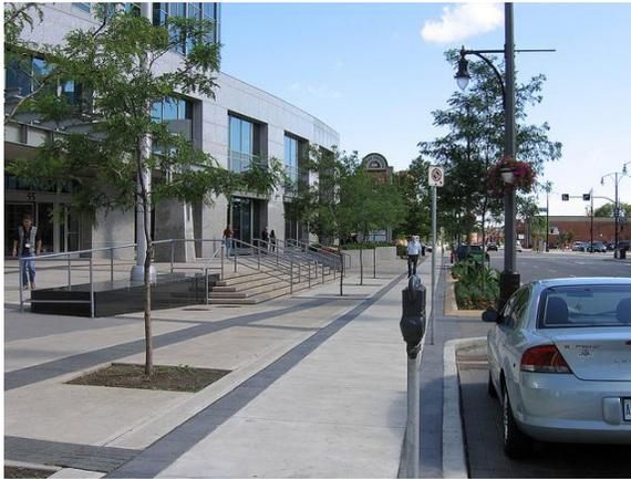
The pedestrian “clear way” is free of obstacles. It is bordered by “shore lines” of darker concrete stamped with a brick pattern providing tonal and textural contrast to the broom-finished concrete sidewalk. All signs, amenities, landscape, etc. are kept outside the clear way.
