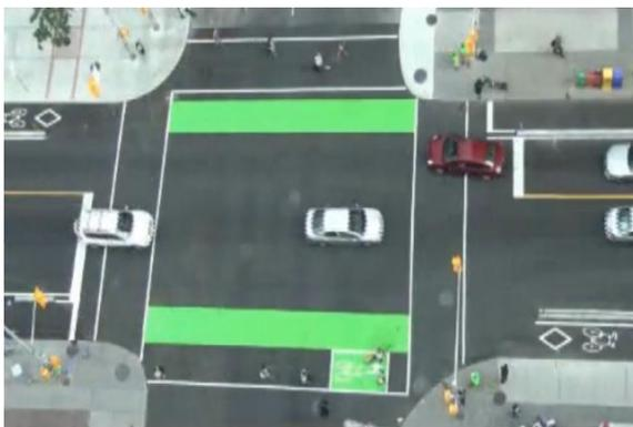
Green pavement, bicycle symbols, elephant's feet and bicycle signals at signalized intersection on a two-way segregated bike lane on a one-way street, Vancouver BC
