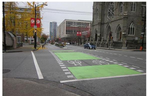
Signalized intersection with left-turn lane, bicycle signals, and segregated bike lane on a one-way street, Long Beach CA
